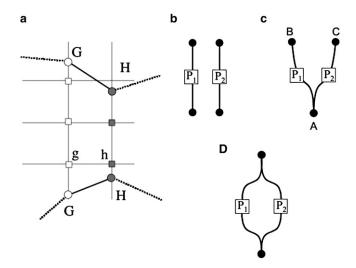
FIGURE 3 (a) Two-dimensional representation of a plug. Shown are the surface (dotted and heavy lines) and the volume grid (light lines). (circles) Bounding vertices G and H, respectively, of the regular A-loop. (squares) The final plug vertices, with fill indicating sides. (b–d) All possible topological cases for a 2-torus: (b) two completely separate pores, (c) two pores that share one endpoint, (d) one pore that bifurcates in the middle.
